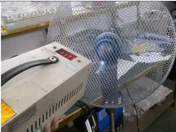
113. Motor rotate speed test for VP65.BL
