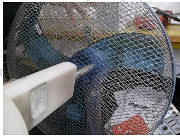
96. Test finger check
