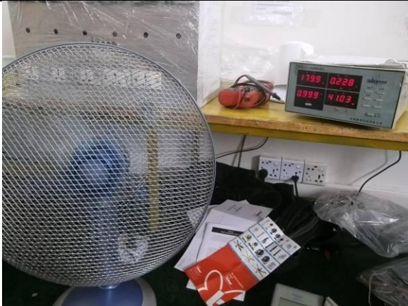
97. Low voltage start test
