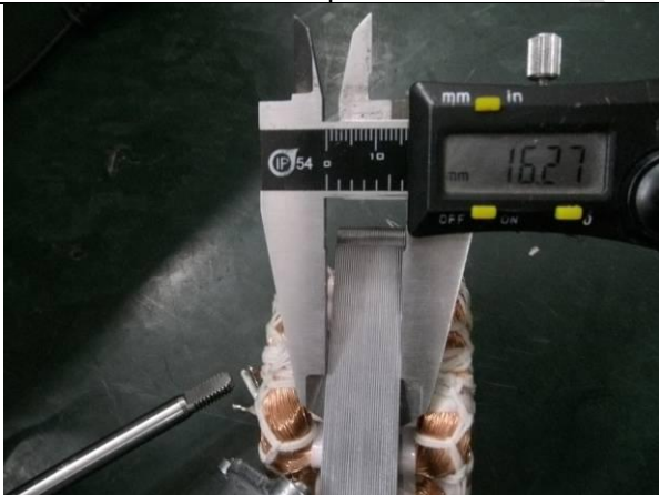
115. Motor size measurement
