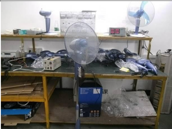
111. Power measurement for VP65.BL
