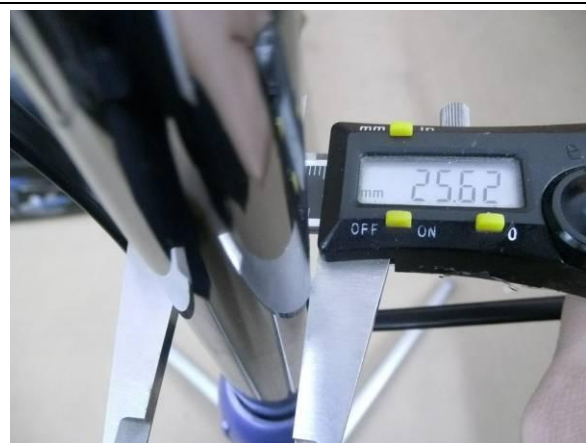
116. Tube size measurement
