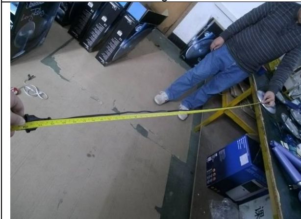
119. Power cord length check
